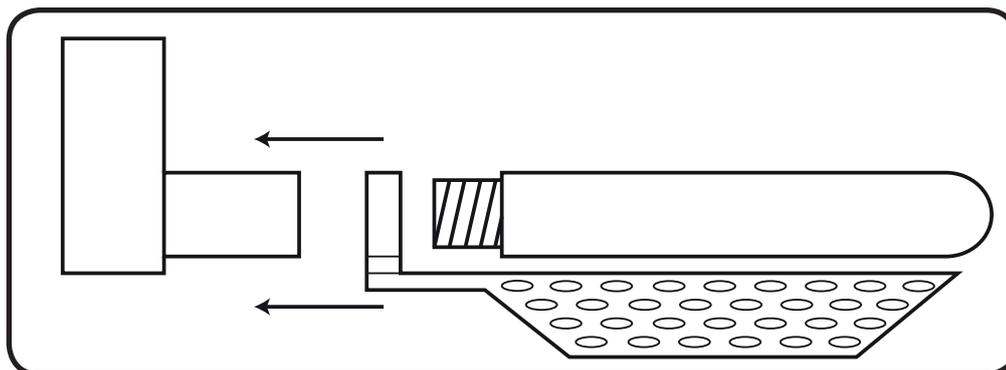
Attaching a Heat Shield to most standard lightholders is simple, as it will easily slide over the ceramic.
