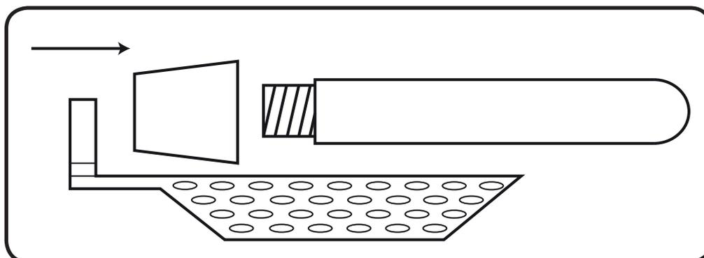
Installing a Heat Shield over conical/flared lightholders is often more difficult due to their shape. It will still fit though! To install on these ceramics, you will need to remove one of the screws at the base of the Heat Shield's circular bracket and then slide it over from the rear. All screws need to be replaced securely after the Heat Shield has been fitted.
