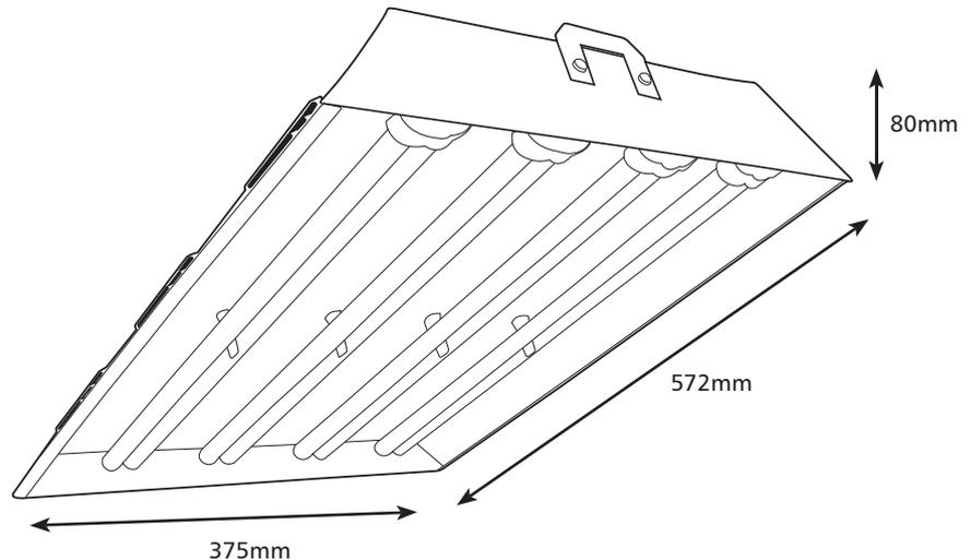
Your Bright-Wing light combines four high output 55 Watt fluorescent tubes and a highly efficient dimpled aluminium reflector to create the ultimate propagation lighting unit. It is ideal for rooting cuttings and seedlings, early vegetative growth or for maintaining a mother plant.
