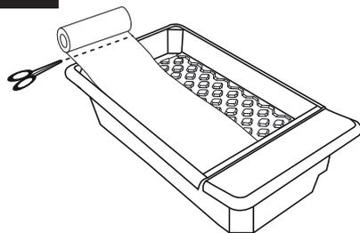
Place a single layer of the spreader mat across the whole of the top tray. This will help to spread the nutrient solution across the whole of the tray where the roots will eventually form.
